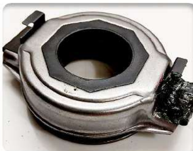
Too much grease
