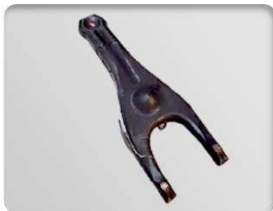
Unable to achieve correct release bearing travel
