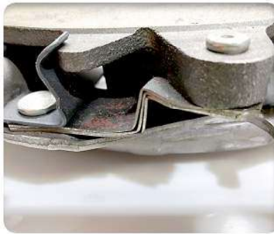
The drive straps of the clutch cover are damaged
