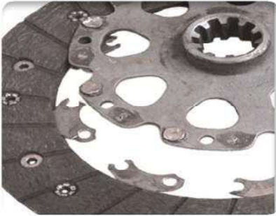
Cushion Plate broken
