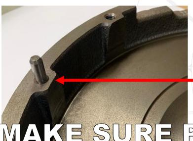
Pressure need to be applied to the disc to clear this section of the flywheel
